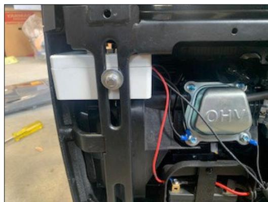
4. Feed the 2 wires on the inner side of the box across to the far side and connect the black to the 'red and black' wire.
