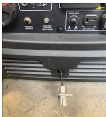
7. Connect the 2 red connectors together and bolt the ring terminal to rocker cover bolt for earth.
