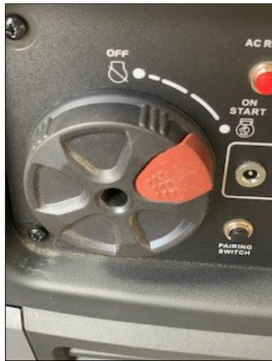
10. After use, make sure the engine switch is turned off, as leaving this in the on position will flatten the battery.
