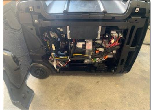
2. Remove the bolts for the front face, there are 4 on the front and 2 from the top and each side.
