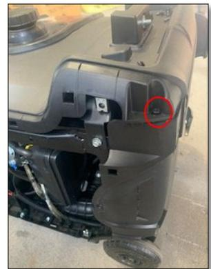
3. Fit the main box as pictured. It is a tight fit and the engine may need to be pushed on the rubber mounts to allow space for the bolt to be fitted into the slot.
