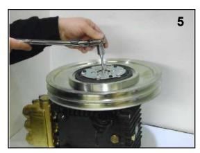
5. Apply anti-seize lubricant to pump shaft. Slide pulley/clutch assembly onto pump. Fasten using bolt with washer. Apply Loctite 243 thread locker to bolt and torque to 8.8 Ft. Lbs.
