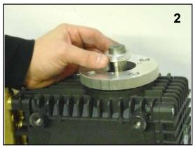
2. Install spacer ring on shaft.
