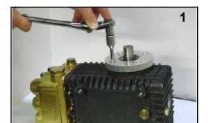
1. Remove four bolts from side cover. Mount adapter plate to pump. Apply Loctite 243 thread locker to bolts and torque to 14.7 Ft. Lbs.
