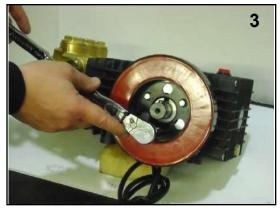
3. Mount coil to adapter plate. Torque bolts to 7.3 Ft. Lbs.
