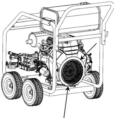
Ensure unit is always run with adequate ventilation and fresh air supply. Do not suffocate engine or obstruct access to cooling fan and intake (see image).
