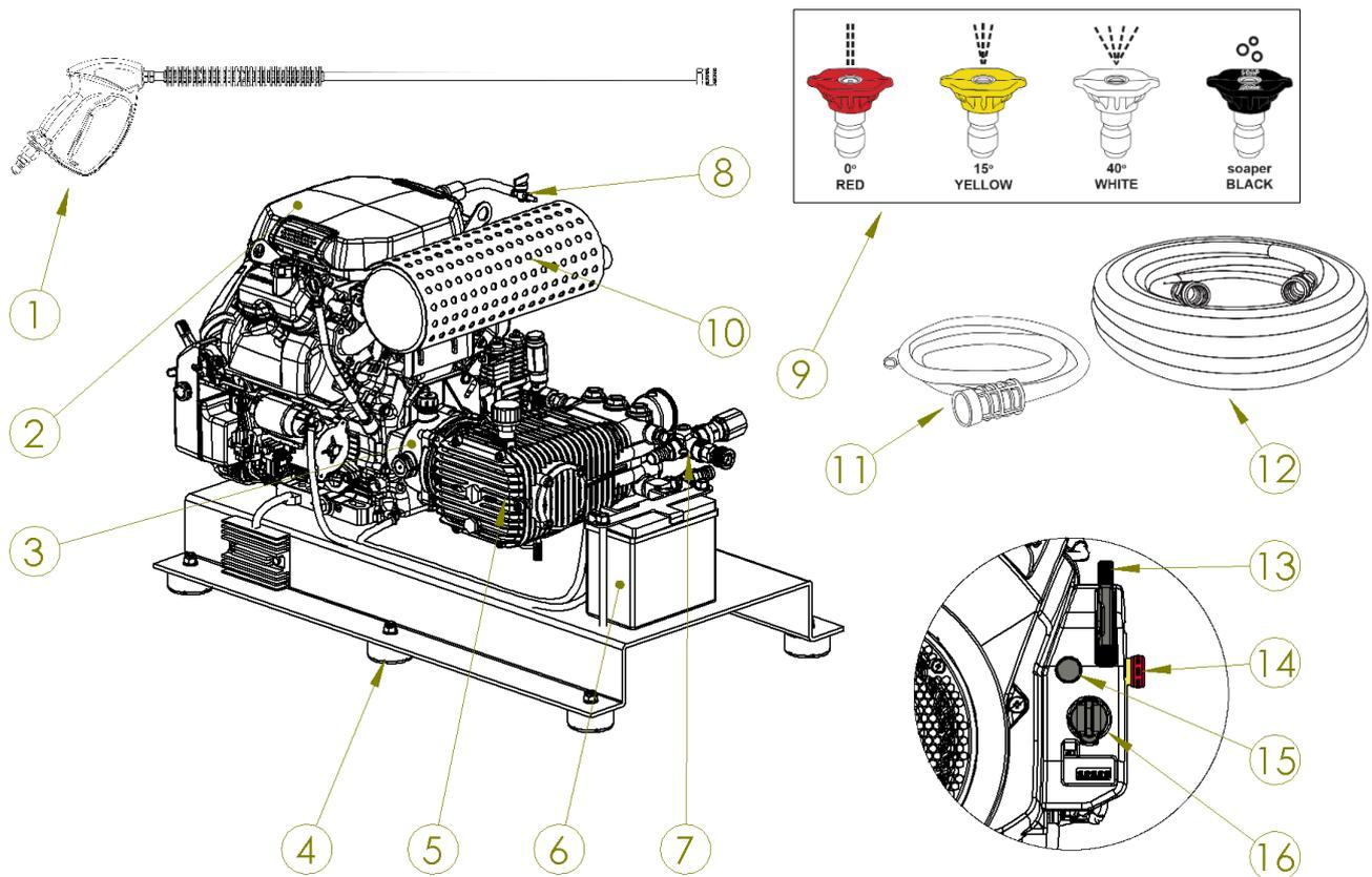
1. **Spray gun/Lance assembly** - Controls the application of water onto cleaning surface with trigger device. Includes trigger lock. Allows you to switch between various spray tips.
