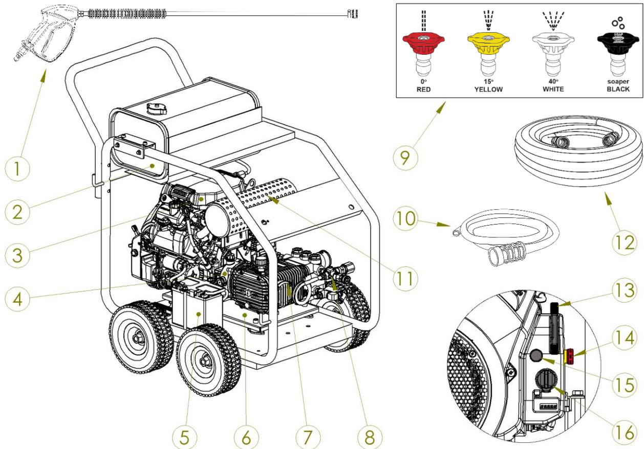
1. **Spray gun/Lance assembly** - Controls the application of water onto cleaning surface with trigger device. Includes trigger lock. Allows you to switch between various spray tips.
