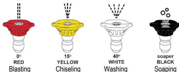
The correct size nozzle will produce maximum pressure at maximum flow. Using an:
