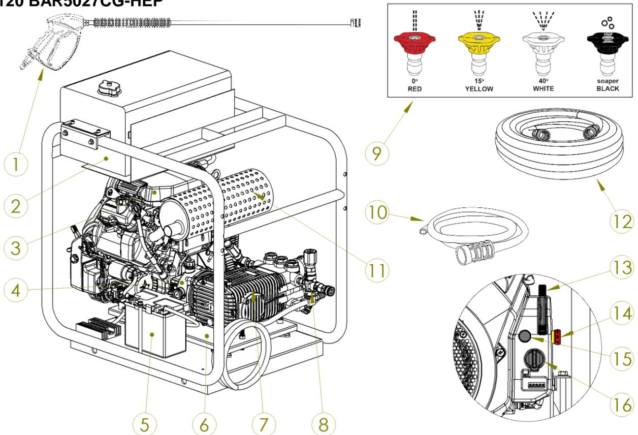
1. **Spray gun/Lance assembly** - Controls the application of water onto cleaning surface with trigger device. Includes trigger lock. Allows you to switch between various spray tips.
